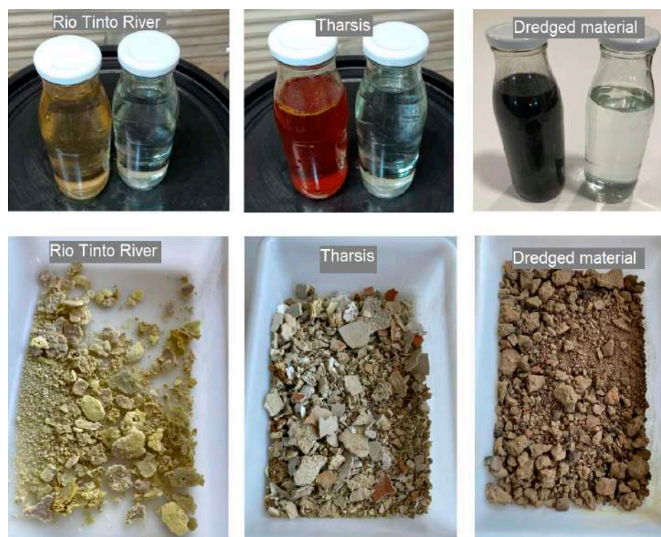
Figure 2. Collected samples (top left) and the treated fluid (top right) from the Rio Tinto river, Tharsis mine and the dredged material. Below are the results in crystallized solids after the treatment with ASEC technology.
